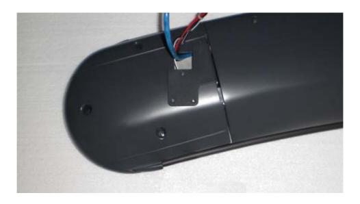
Locate the two support columns and the six M3 X 6mm screws, washers and star washers.
