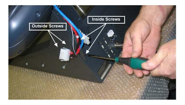
When all the screws are in place, tighten each of them. Repeat this step for both sides of the console.
