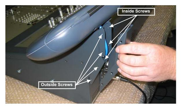
When all the screws are inserted, tighten each of them.
