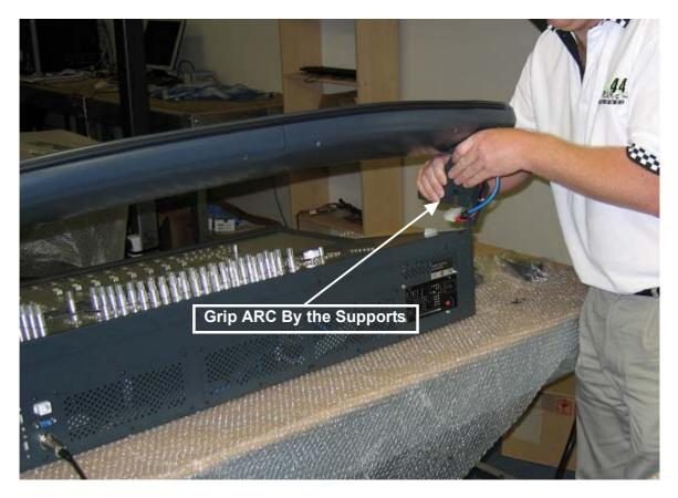
Once the **ARC** is aligned, carefully lower it into position and continue to support it while the fixing screws are inserted and tightened.
